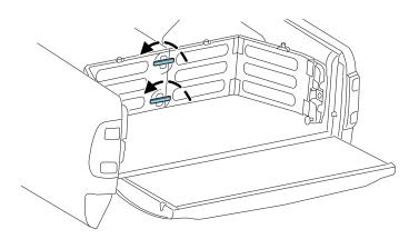
To open the bed extender into Grocery Mode, follow Steps 1–5 by rotating the panels away from the tailgate.
